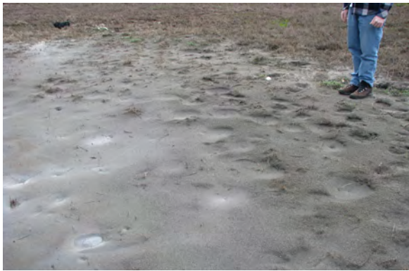
Liquefaction features. Left – remains of sandboils at Centerville Beach. Right – sandboil along the Eel River.
