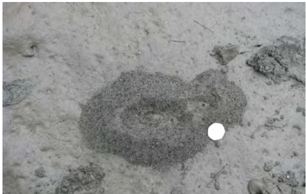
Liquefaction features. Left – remains of sandboils at Centerville Beach. Right – sandboil along the Eel River.
