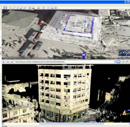
Cal balloon → Interactive panoramic movie of Ascotia Hotel & its surrounding & interactive image with links to points clouds from the laser scanner (TruView) to perform any measurements of the objects
